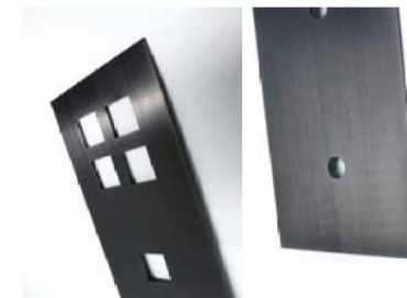
Figure 1: deposition on Steel 3D parts
